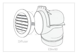
Installation using Primex's 'Squeeze Elbow'
