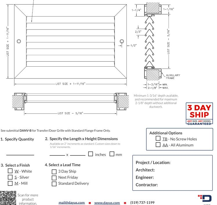
INVERTED V BLADE ON 2/3" SPACING
