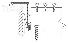
Product is fastened to duct-mounted brackets, which are concealed behind the blades.
